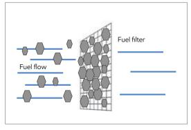
Wax separates from untreated fuel and creates rhombic wax crystals that rapidly cover the filter.
