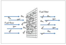
Cold-flow improver modifies the wax crystals into needle-shaped crystals, allowing some wax and fuel to pass through the filter.
